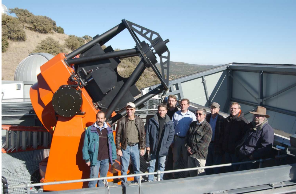
Fig. 1. The MONET/North telescope at its final site at McDonald Observatory in Texas during installation in December 2005. One half of the wide opened clam-shell enclosure is seen to the right; one can also notice that the sky is nearly unobstructed by the enclosure. The installation team from University of Göttingen, McDonald Observatory, and Halfmann Teleskoptechnik is celebrating the first successful tests.
